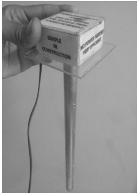
Figure 1: Self-made capacitance probe
