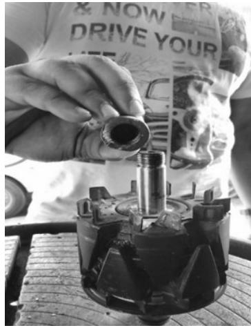
Fig 8: Field of an alternator
