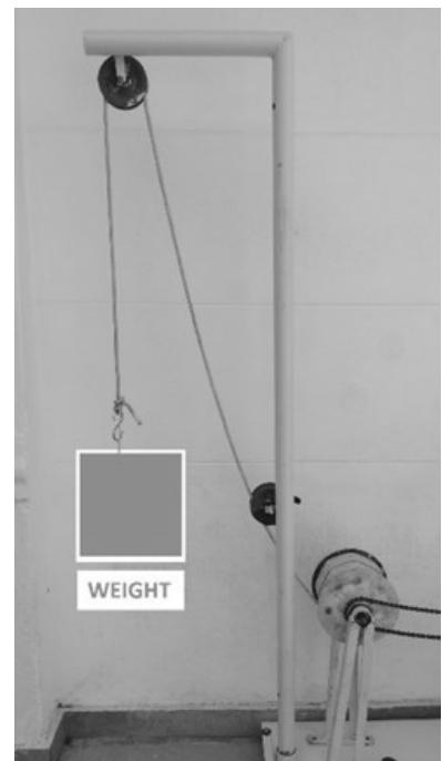
Fig 5: Rope, drum and load arrangement
